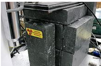
Gamma radiation has such a high penetrating power you need a very thick barrier to stop it.
