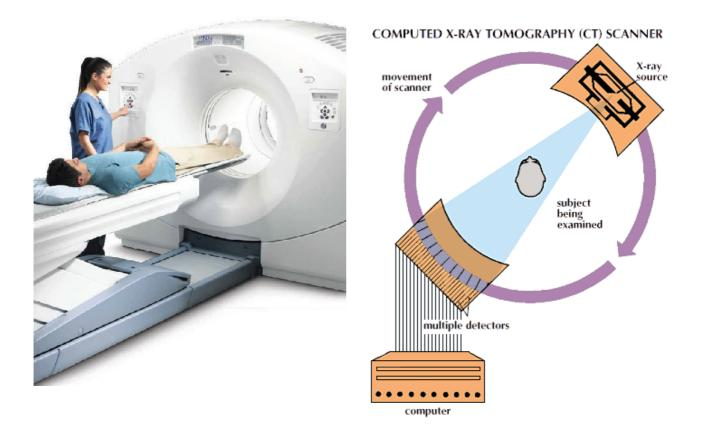
In many industrial CT scanners that use physically larger sources and detectors, and typically analyse smaller samples (with greater precision) it becomes far easier to simply rotate the sample.
